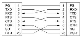
Using crossover cable with D-SUB 9-pin and 25-pin connectors
